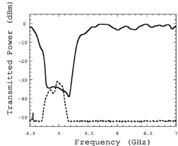
FIG. 3. A transmission experiment for the case of  $H_{\parallel}$ . The upper curve (solid line) is that of the SRR array with lattice parameter  $a = 8.0$  mm. By adding wires uniformly between split rings, a passband occurs where  $\mu$  and  $\epsilon$  are both negative (dashed curve). The transmitted power of the wires alone is coincident with that of the instrumental noise floor ( $-52$  dB).
