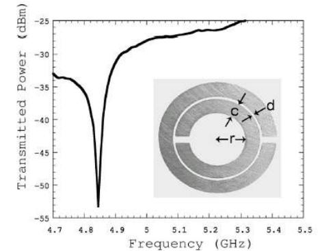
FIG. 1. Resonance curve of an actual copper split ring resonator (SRR).  $c = 0.8$  mm,  $d = 0.2$  mm, and  $r = 1.5$  mm. The SRR has its resonance at about 4.845 GHz, and the quality factor has been measured to be  $Q = f_0/\Delta f_{3dB} > 600$ , consistent with numerical simulations.
