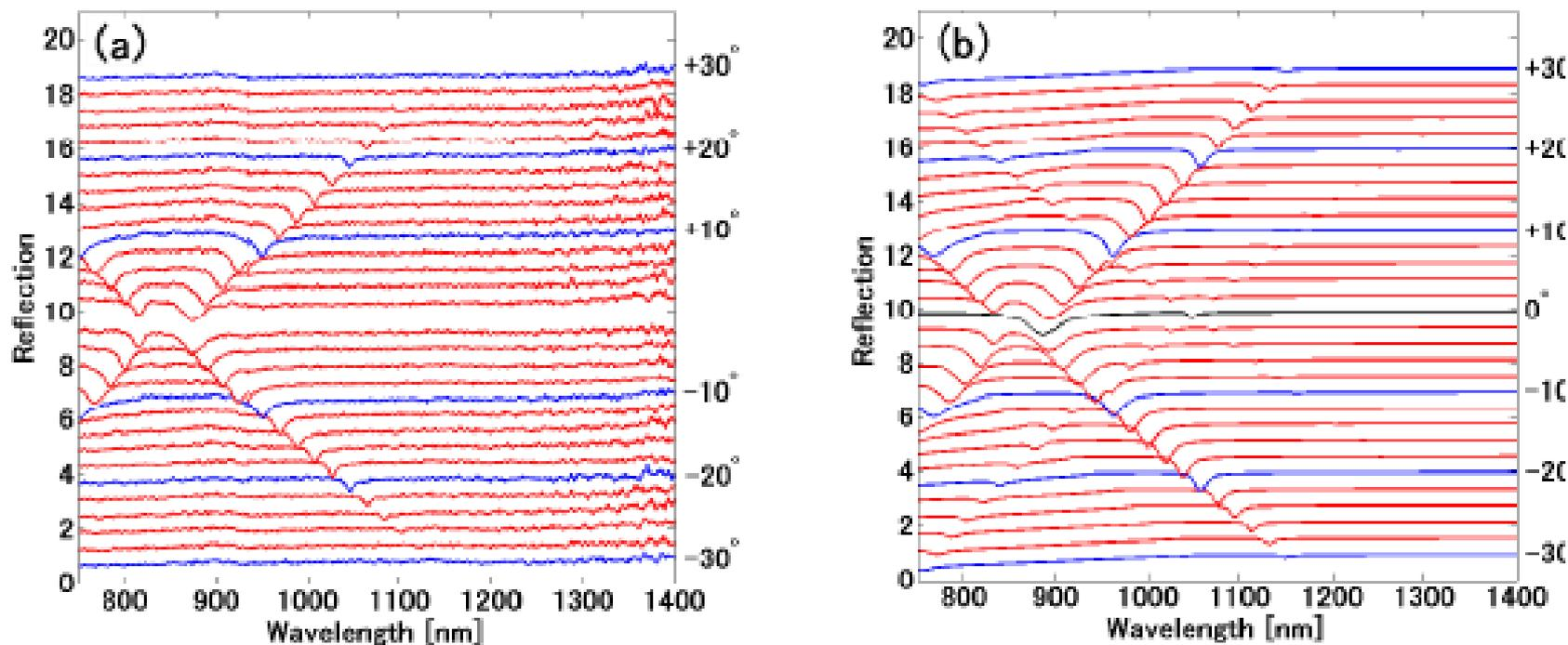
Fig. 2. (a): Experimental result of reflection spectra. (b): Numerical calculation of reflection spectra.
