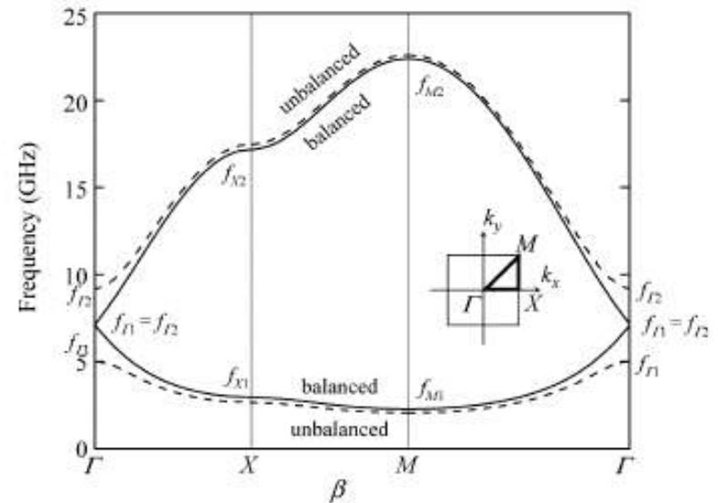
Fig. 5. Dispersion diagram of the structure. Solid line: balanced case ( $L_L = 1.0$  nH,  $C_L = 0.5$  pF,  $L_L = 1.0$  nH,  $C_L = 0.5$  pF). Dashed line: unbalanced case ( $L_L = 0.6$  nH,  $C_L = 1.0$  pF,  $L_L = 1.0$  nH,  $C_L = 0.5$  pF). The  $\Gamma$ ,  $X$ , and  $M$  represent the high symmetry points ( $k_x a = k_y a = 0$ ), ( $k_x a = \pi$ ,  $k_y a = 0$ ), and ( $k_x a = k_y a = \pi$ ), respectively in the spectral domain.
