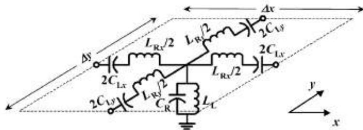
Fig. 4. Equivalent circuit of the unit cell of the 2-D CRLH TL.
