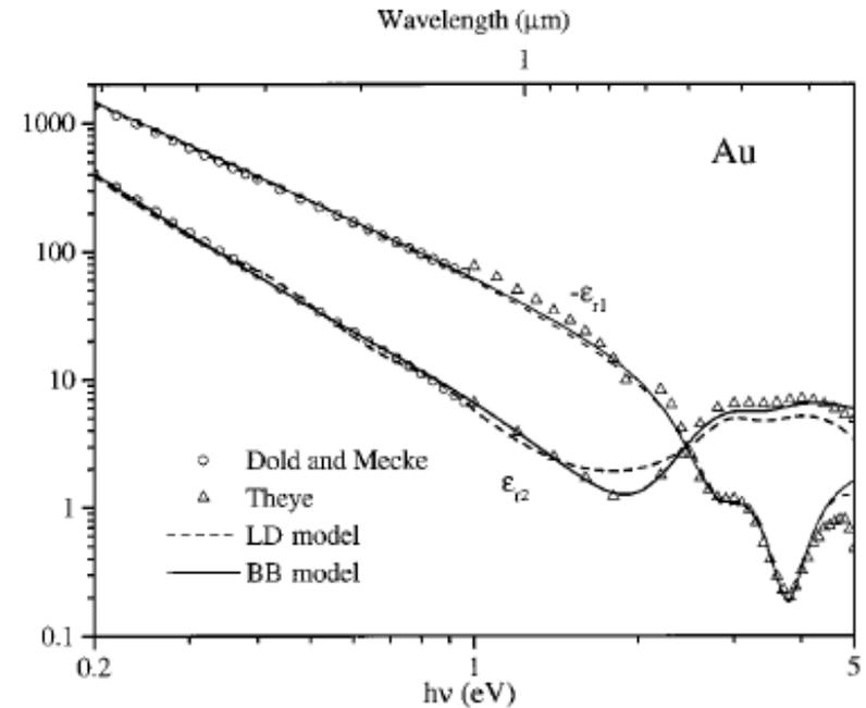
Fig. 2. Real and imaginary parts of the optical dielectric function of Au: solid curves, values that we calculated using the BB model; dashed curves, the LD model. Also shown are selected experimental data points from Dold and Mecke<sup>46</sup> and Theye.<sup>49</sup>
