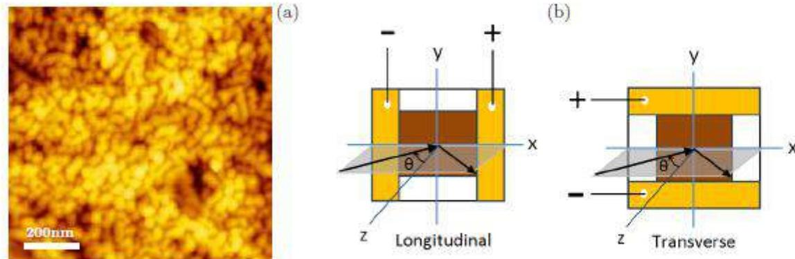
Fig. 1. (a) AFM image of NPG film shows that it is a network of pores and gold. (b) Two configurations for measuring PIV in NPG. The arrow shows definition of the positive incident angle ( $\theta$ ) in the configurations.
