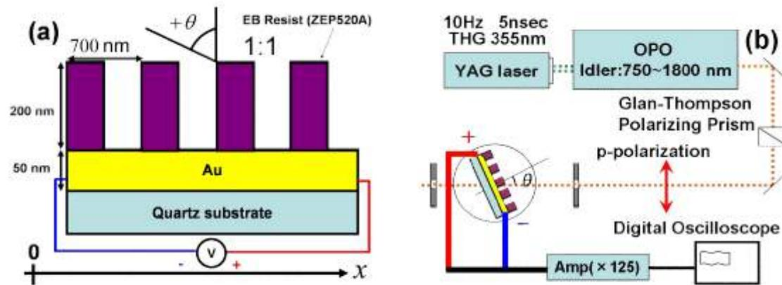
Fig. 1. (a): Schematic of the structure. (b): Experimental setup.
