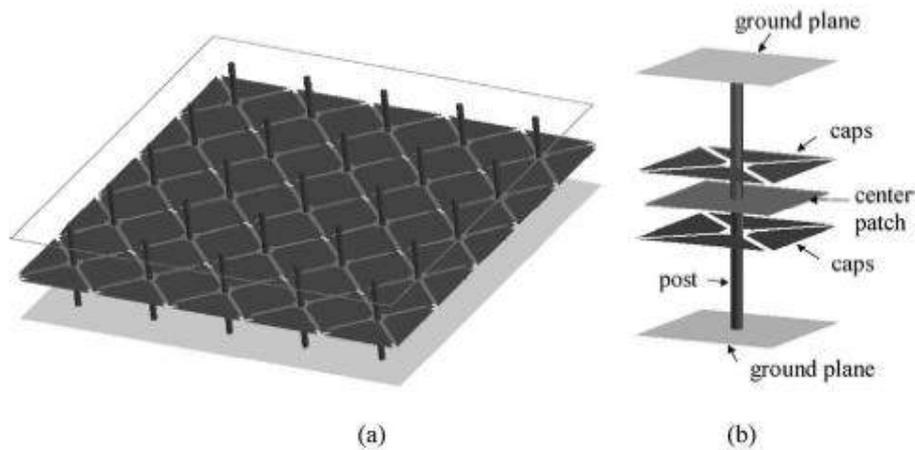
Fig. 3. Closed (stripline) structure. (a) General view. The top ground plane is drawn transparently for easy view. (b) Unit cell.
