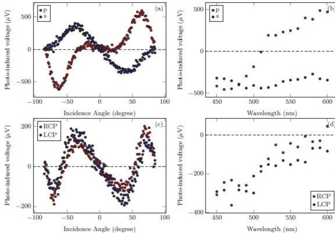
Fig. 5. (a) Angle resolved LPIV for 580 nm, p- and s- polarized light. (b) Wavelength resolved LPIV for +50° incidence angle, p- and s- polarized light. (c) Angle resolved LPIV for 580 nm, circular polarized light. (d) Wavelength resolved LPIV for +50° incidence angle, circular polarized light.
