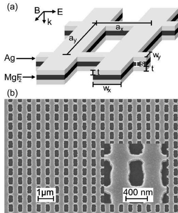
Fig. 1. (a) Scheme of the negative-index metamaterial design and polarization configuration. The sample parameters used in Figs. 2 and 3 are given:  $w_x=316$  nm,  $w_y=100$  nm,  $t=45$  nm,  $s=30$  nm, and lattice constant  $a_x=a_y=600$  nm. (b) Top-view electron micrograph of the silver-based structure. Inset, magnified view.
