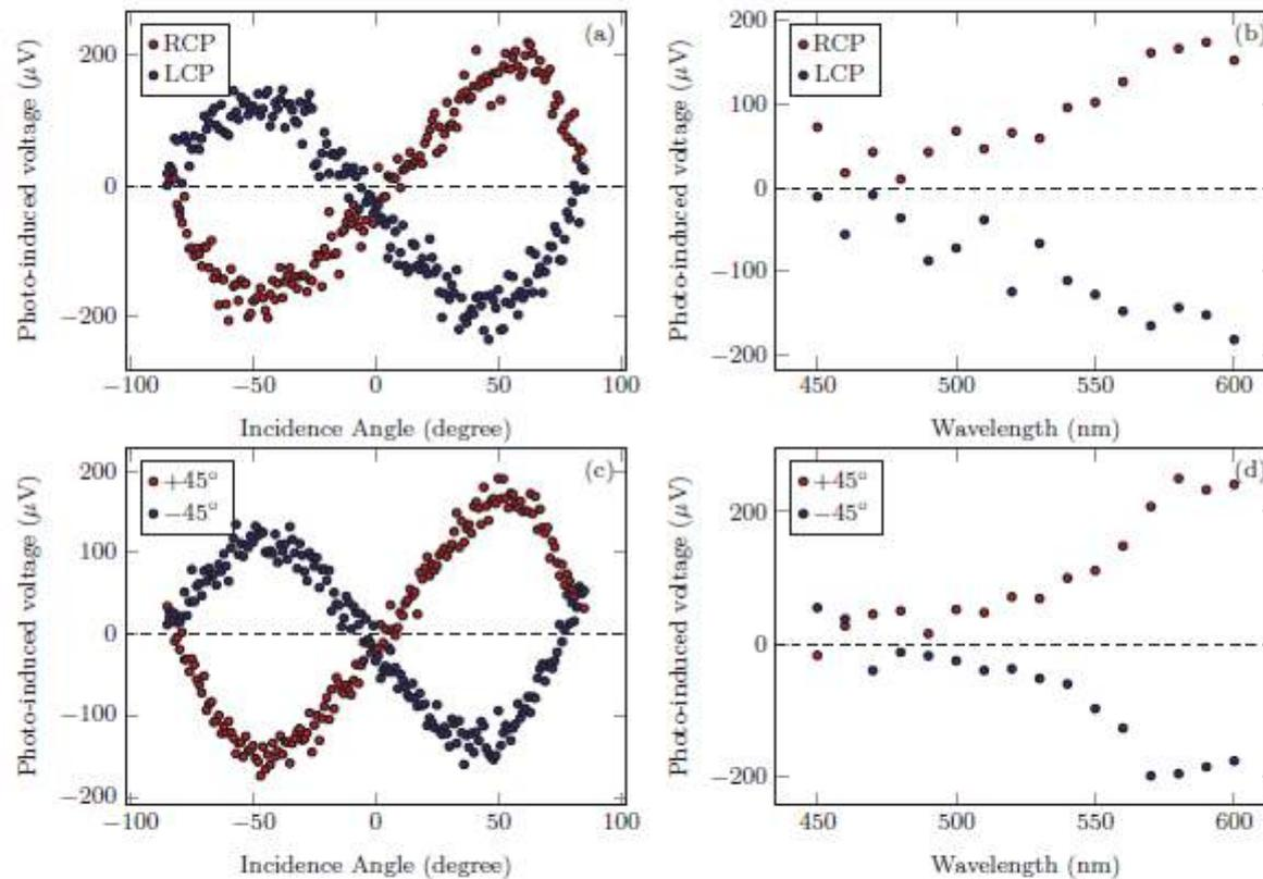
Fig. 4. (a) Angle resolved TPIV for 550 nm, circular polarized light. (b) Wavelength resolved TPIV for +50° incidence angle, circular polarized light. (c) Angle resolved TPIV for 550 nm,  $\pm 45^\circ$  linear polarized light. (d) Wavelength resolved TPIV for +50° incidence angle,  $\pm 45^\circ$  linear polarized light.
